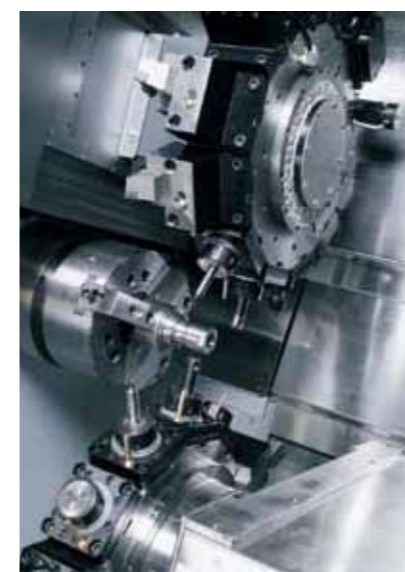
● Upper/ lower simultaneous Y-axis milling on the left hand side
