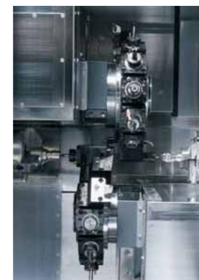
● Upper-right/ lower-left axial milling operation
