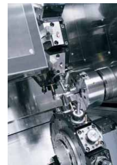
● Upper/ lower simultaneous Y-axis milling on the right hand side
