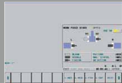
● Work-piece statement display Display for machines with Gantry Loader.
