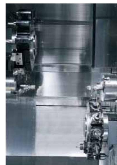
● Upper-left/ lower-right radial milling operation
